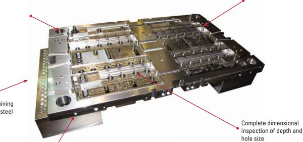
Complete machining of all alloy tool steel
